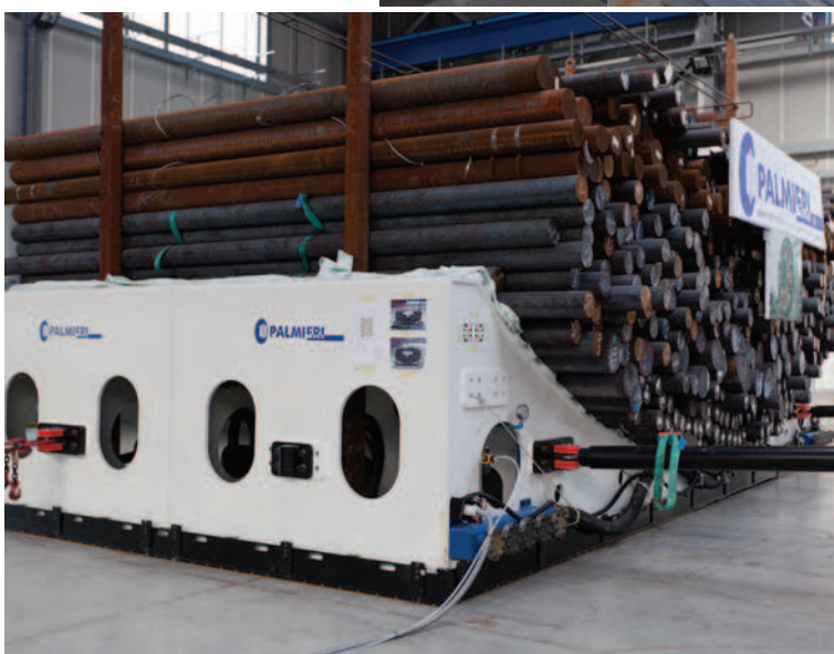
Bottom: Testing the air cushion frame
